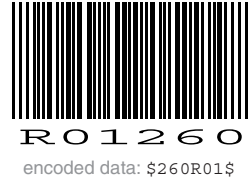
Fig. C.20. Example for Codabar
