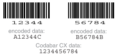
Fig. C.22. Example for Codabar CX
