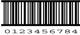
Fig. C.24. Example for Interleaved 2of5 with bearer bars
