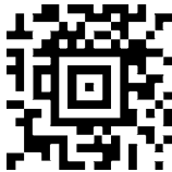
Fig. C.46. Example for Aztec
