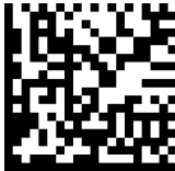
Fig. C.45. Example for DataMatrix (ECC200)
