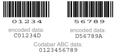
Fig. C.21. Example for Codabar ABC
