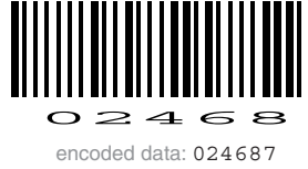
Fig. C.30. Example for MSI/Plessey with MOD 10 Checksum
